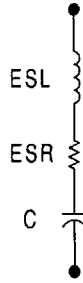
Figure 2-12: Lumped parameter circuit model of a real capacitor. ESL is the equivalent series inductance and ESR is the equivalent series resistance of the capacitor leads. These parasitic elements make the capacitor look inductive or resistive at high frequencies.
