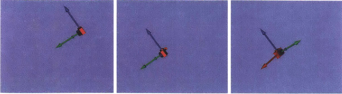
Figure 2-7: This shows translation and rotation in the local coordinate system of the camera: the endoscope is at an initial position on the left screen, on the middle screen, the endoscope has been translated along its x (green) axis and on the right screen, the endoscope is then rotated along its z (blue axis).
