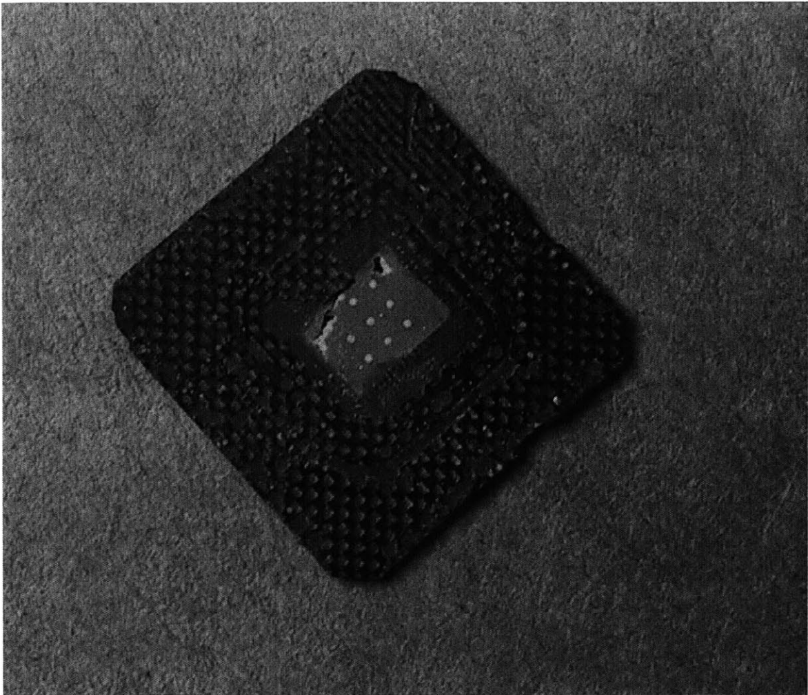
Figure A-5: Top Portion of the Package, the Light Green Area is the Back Side of the Die
