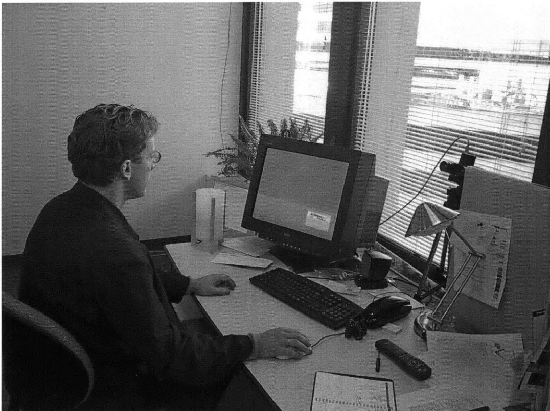
Figure 5-2: A user is sitting at his desk (his local presence display monitor in the back is green) and the person he is remotely connected to is currently busy (the lamp is red).
