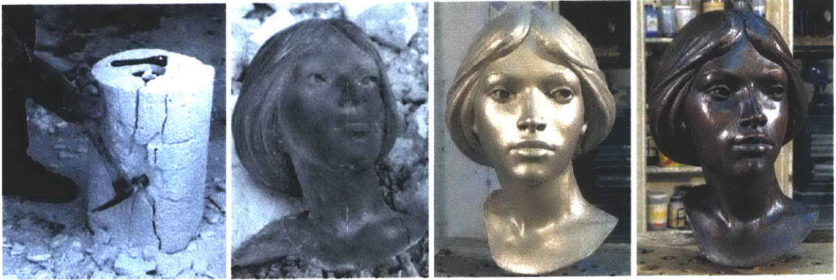
Figure 10.7: These photographs of the lost wax casting process from Llangland [1999] follow the process after the stages illustrated in Figure 10.6. The outer layer of clay is broken away with a hammer to reveal the sculpture. After polishing and sandblasting, the raw metal is bright and shiny. Different chemicals are applied to the sculpture to achieve a particular patina and the model is sealed with a coat of wax.
