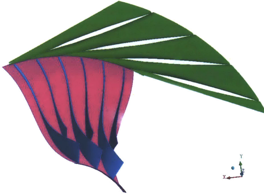
Figure 3-12: Schematic of the research centrifugal compressor stage CFD domain, adopted from Gould [9].
