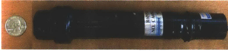
Figure 4-5: An image of the EJ301-PMT detector next to a U.S. quarter for scale. The slightly bulging cylinder at the left contains the EJ301 liquid scintillator in an aluminum canister; the majority of the detector is the 1 inch diameter PMT.
