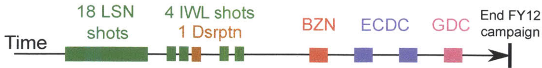
Figure 7-1: A timeline illustrating the plasma operations and wall conditioning processes that were carried out during the end of the FY12 Alcator C-Mod experimental campaign. The GDC was the final PFC perturbing process before the vacuum vessel was brought up to air for the maintenance period.
