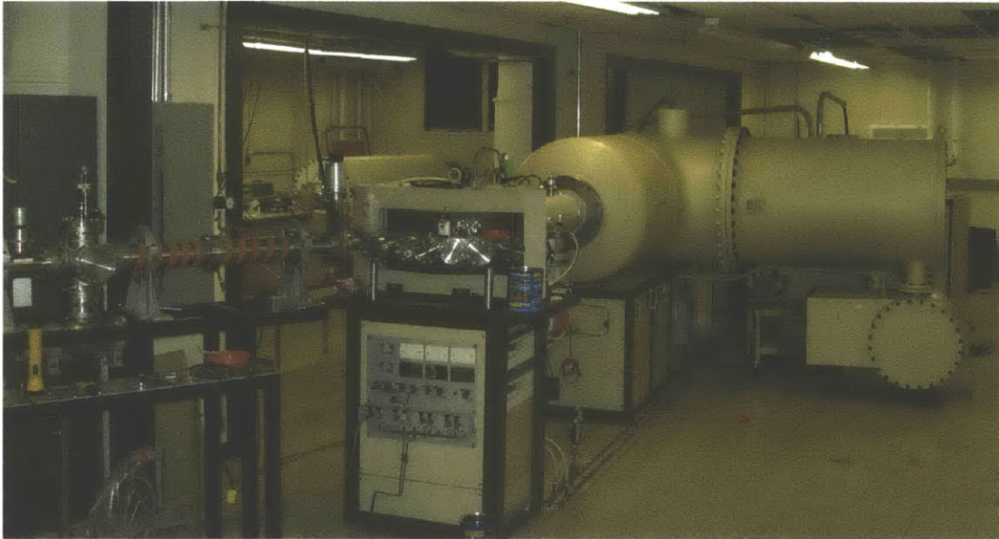
Figure 3-1: Photo of the 1.7 MV tandem accelerator in the CLASS facility
