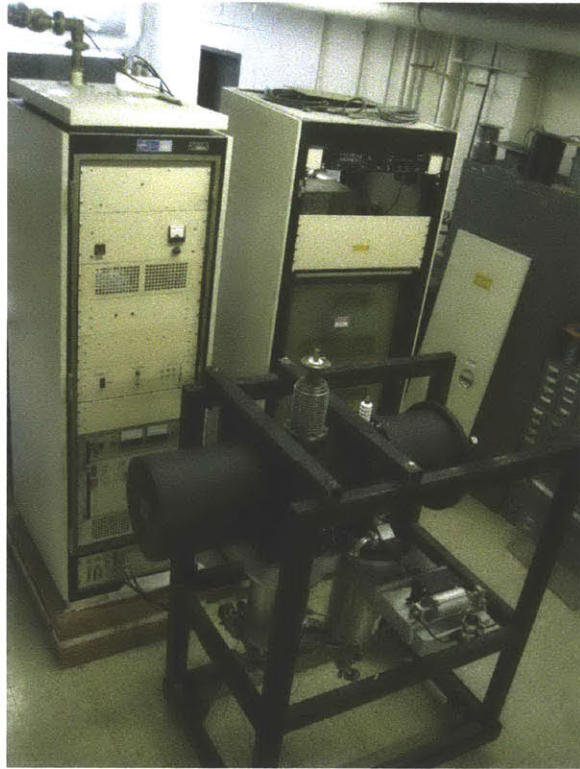
Figure 4-6: RFQ accelerator (black) with 60 kW amplifier (upper left) and ion source power supply and control rack (upper right).
