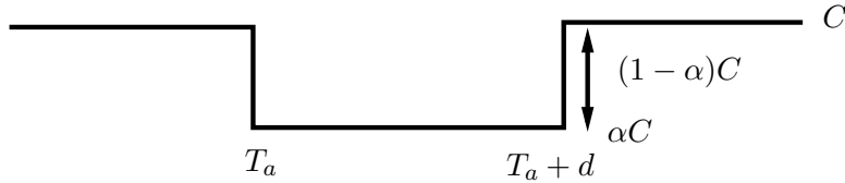
Figure 3: Depiction of the capacity profile under a weather-front based uncertainty set for a single affected airspace element. The plot is for a particular realization of the parameters (T_a, d, \alpha) .
