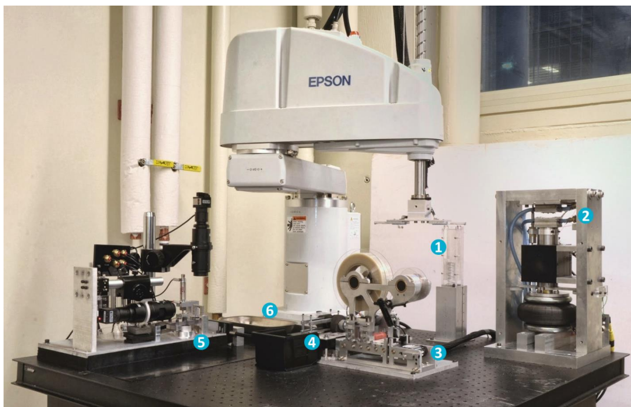
Figure 7-1: The complete microfactory system with labeled stations. (1) Spring-loaded dispenser with blank chips. (2) Hot embossing machine. (3) Taping machine. (4) Cutting station. (5) Functional testing machine. (6) Tray for collecting tested chips.
