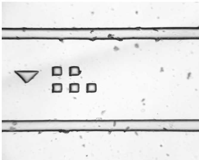
Figure 4-2: A micrograph of a chip sealed with Tesa Tape 62551.
