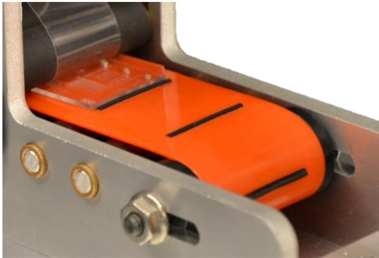
Figure 4-9: First prototype of the belt. A bolt and nut were used on the front roller to apply tension.
