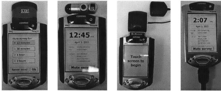
Figure 4-4: These images show the Context-Aware Experience Sampling Tool with sensors: The bar code scanner (left) can read standard 2D bar codes. The camera (left-center) enables subjects to take a picture as an alternate answer to questions when enabled by the researcher. The GPS receiver (right-center) provides outdoor location data. The iPAQ serial cable (right) enables CAES to support for a wide range of sensors, such as a wireless Polar heart rate monitor.
