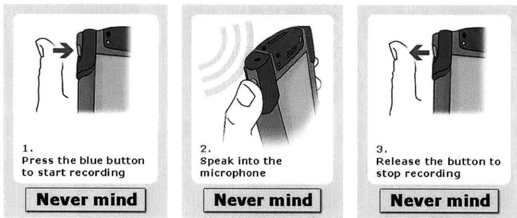
Figure A-7: These Help screens are rotated on the screen every couple seconds when the subject selects the Attach audio note option on the Question screen. These screens are displayed until the subject activates the microphone or they select Never mind . If the subject activates the microphone the appropriate Device screen is displayed. If the subject selects Never mind they are returned to the Question screen without attaching an audio note.
