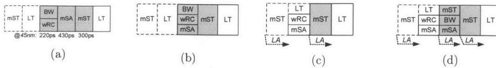
Figure 4-8: FANOUT pipeline optimizations to realize single-cycle multicast router: (a) 3-stage pipeline, (b) 2-stage pipeline, (c) 1-cycle pipeline (with bypass), (d) 2-stage pipeline (if bypass fails)
