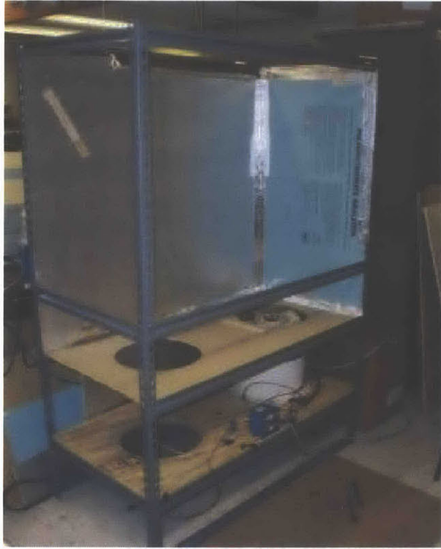
Fig. 3-16: Single housing used to enclose two ventilation fans.
