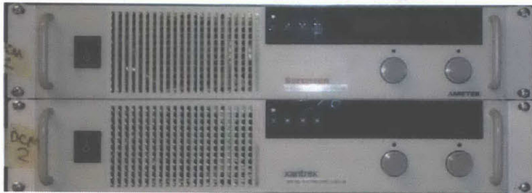
Fig. F-4: DC power supplies. 150 Vdc and 18 A and 2700 W
