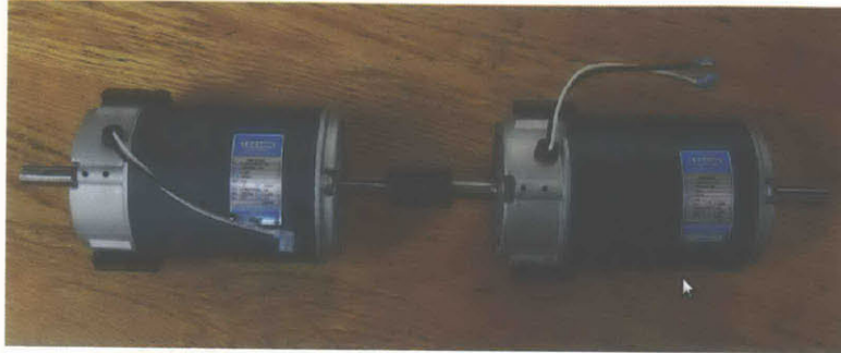
Fig. F-3: Coupled permanent magnet DC motors used as prime movers [101].
