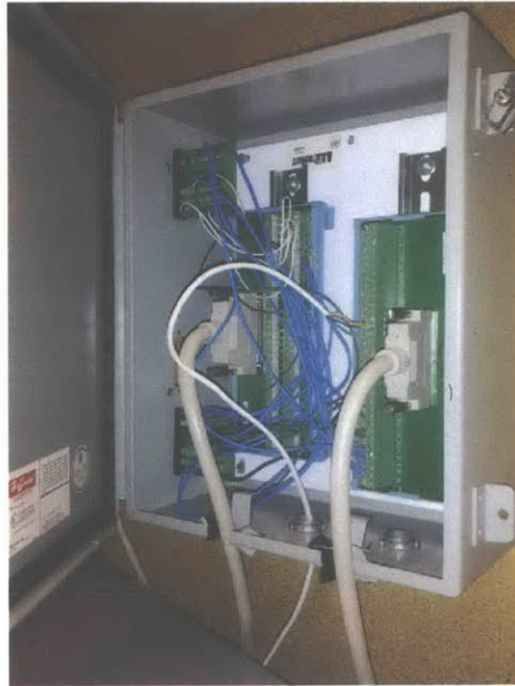
Fig. F-10: SCSI terminal blocks are used to connect the PCI-1710 cards with external components.
