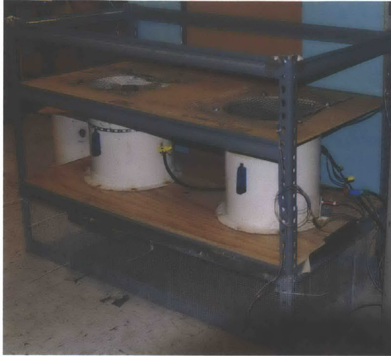
Fig. 5-1: Laboratory setup with two ventilation fans mounted to a steel frame.
