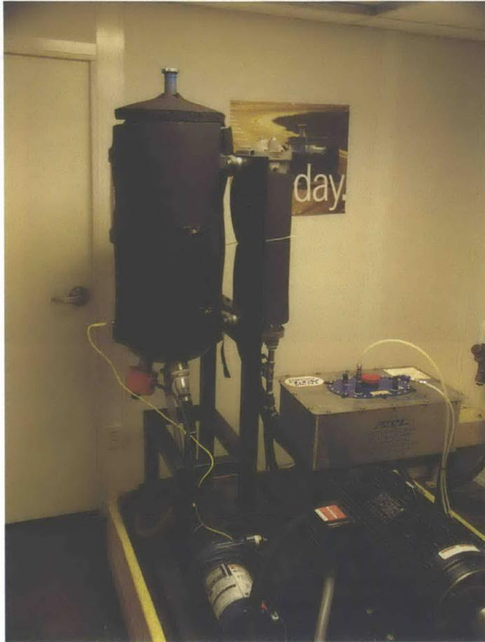
Figure 3-26: Engine cooling reservoir, heat exchanger, and pump.
