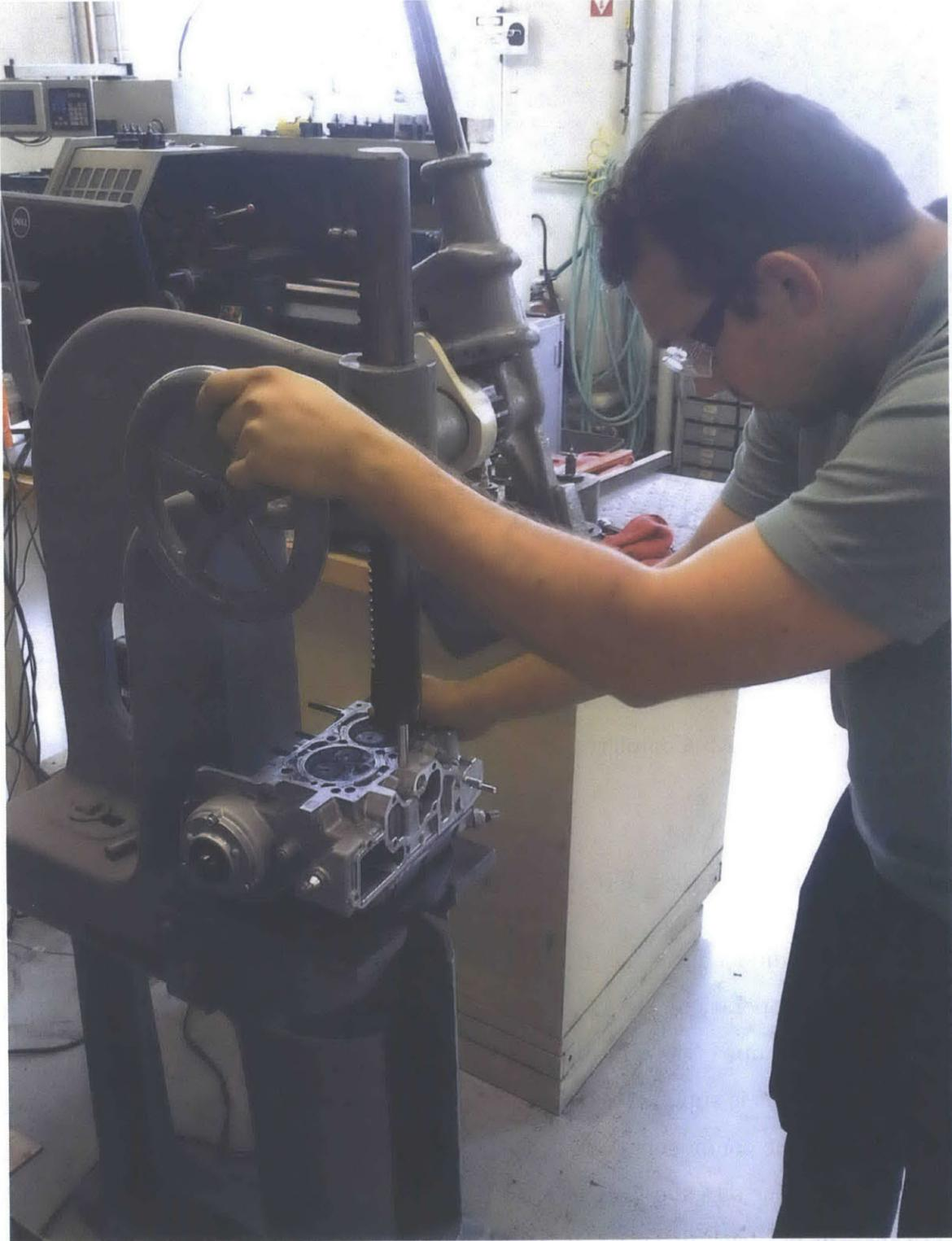
Figure 3-23: Installation of stock lubrication passage interference plugs to separate the lubrication circuit.
