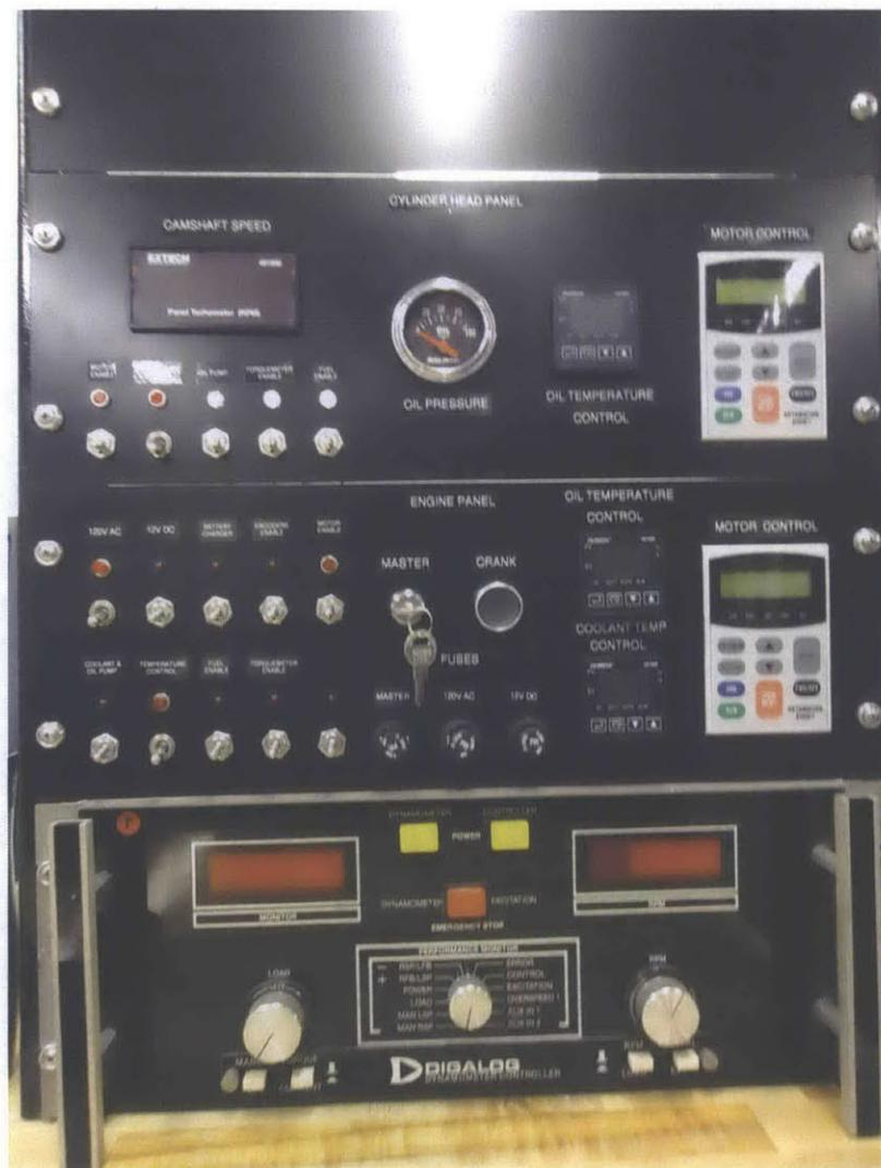
Figure 3-28: Operator instrument control panel.
