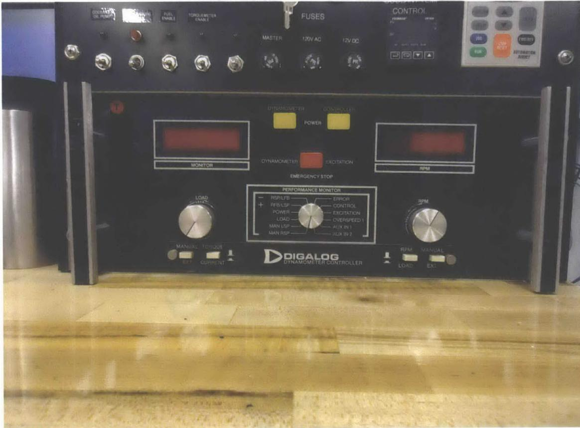
Figure 3-5: Dynamometer controller - Digalog Series 1000A
