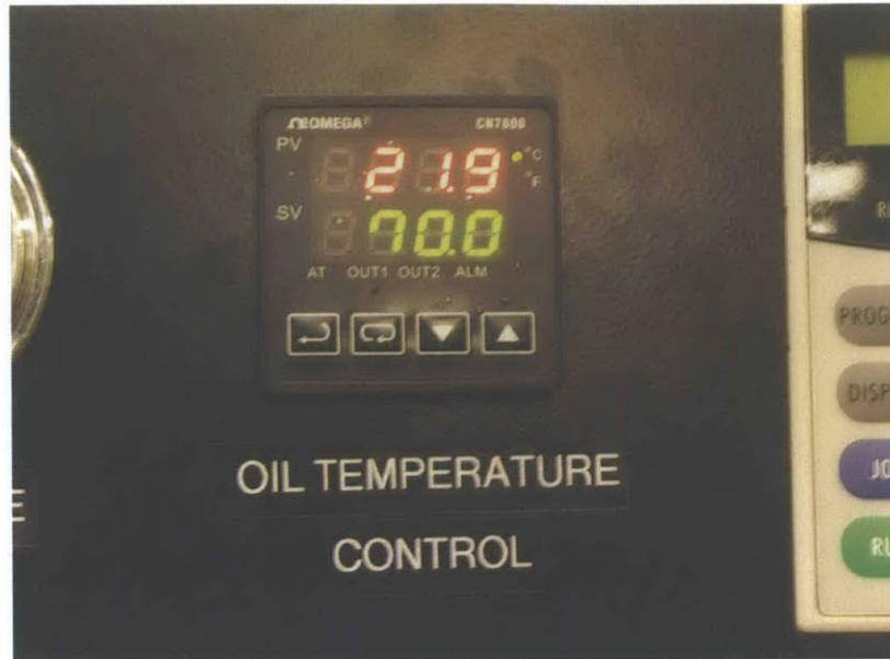
Figure 3-25: Omega CN7800 temperature controller.
