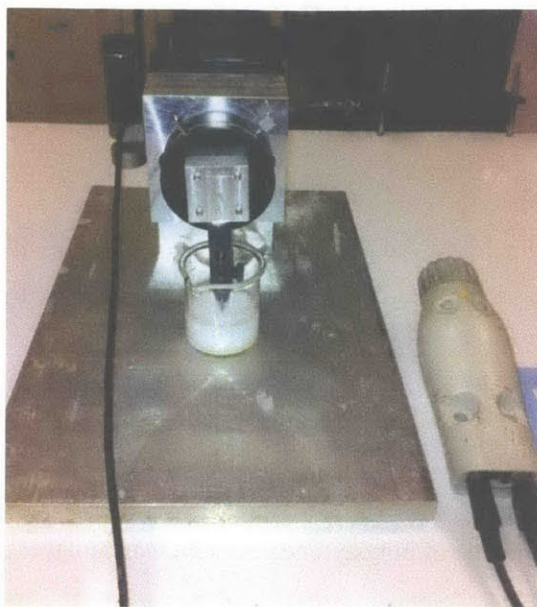
Figure 2.4 Dip coating process. The device used is a custom-built dip coater.
