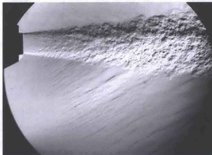
Figure 5.5: Unprocessed Schlieren image showing the presence of Mach wave radiation as reproduced from Pappaschou [51]. The individual Mach waves can be observed clearly from this representative, unprocessed Schlieren image.
