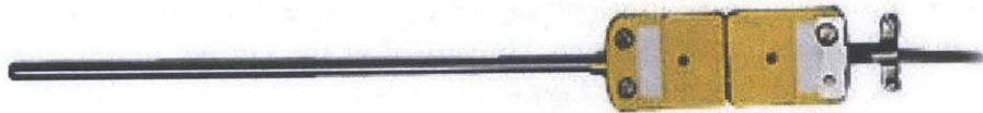
Figure 2.9.2: Photograph of a typical K-type thermocouple probe. This particular probe shows a grounded style tip. The type of thermocouple used in these experiments was the exposed tip thermocouple type, allowing for faster response.
