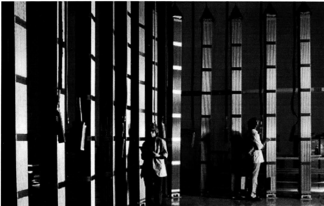
Figure 7 Westinghouse PWR fuel assemblies [Ref. 14]
