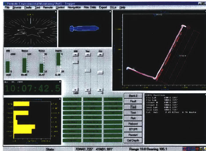
Figure 3-2: Windows based Graphical User Interface for the REMUS vehicle. This program allows programming missions and downloading mission data when the vehicle is connected to a laptop or modem. Photo courtesy of WHOI OSL.
