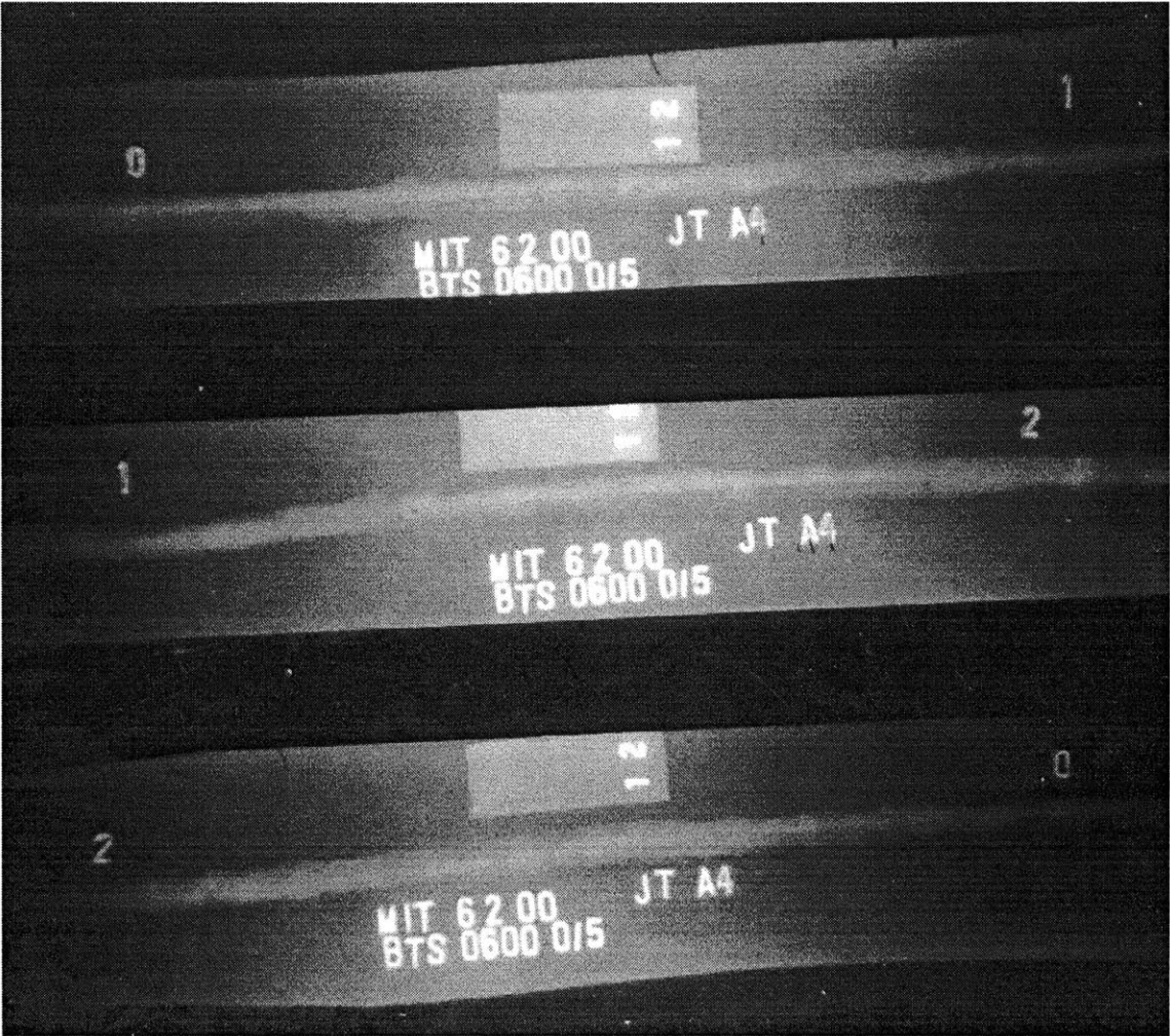
Figure A-4: Weld A4 Before Repair
