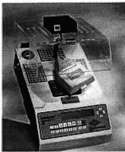
Figure 6-1: The Robocycler Gradient 96: the machine used for the positive controls in the 30 cycle experiments. The Robocycler has a robotic arm that moves the tubes between 4 different temperature heat blocks (denaturing, annealing, extension, and refrigerated storage). From [83].
