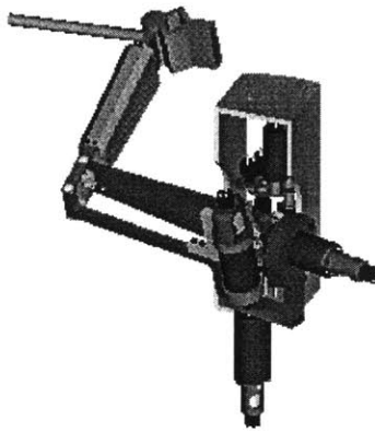
Figure 2-2. 3 DOF "Linear Haptic Display" by haptic technologies Inc.
