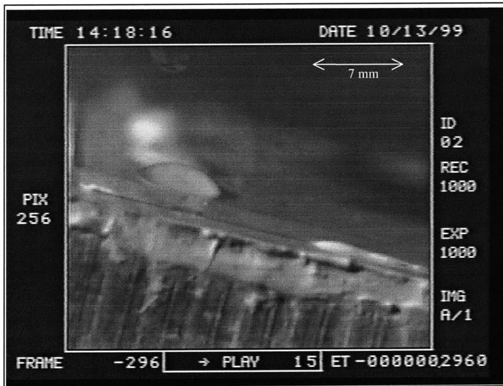
Figure 3.2 - Deposition on a plate inclined at 15^\circ HSC S=0.19 , \gamma=15 (Run 367) after complete arrest, but before completion of bulk solidification
