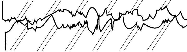
Figure 5-2: Contact between two solid bodies is limited to the contact of small protuberances called asperities.
