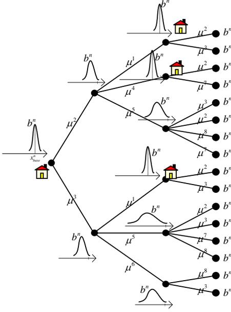
Fig. 3. Illustrates the search tree in the non-stabilizable belief space for the depth of three (corresponding to the graph in Fig. 2). Taking edges  $\mu^1$  and  $\mu^4$  drives the system to recharge stations, where the non-stabilizable belief gets reset.
