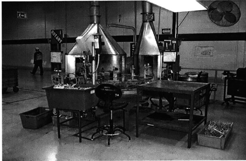
Figure 1.12: Rotary brazing machine used for aluminum parts
