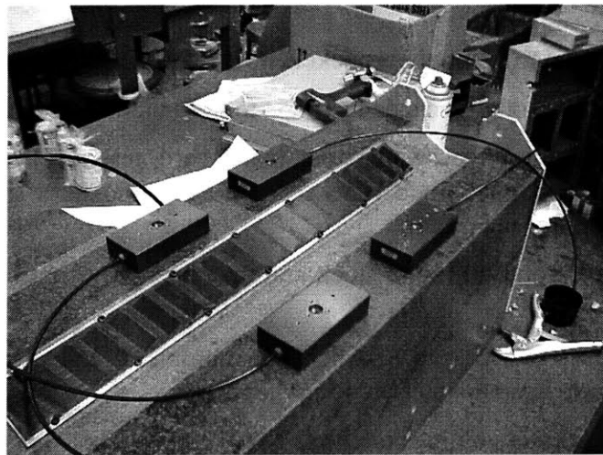
Figure A.5 The top bearings in their approximate locations on the Way.
