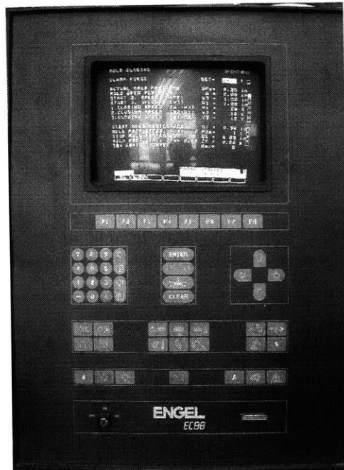
Figure 6.4: Injection Molding Machine controller panel
