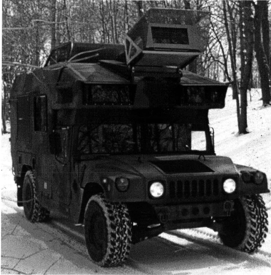
Figure 8: The CMU Unmanned Ground Vehicle Navlab II [20].
