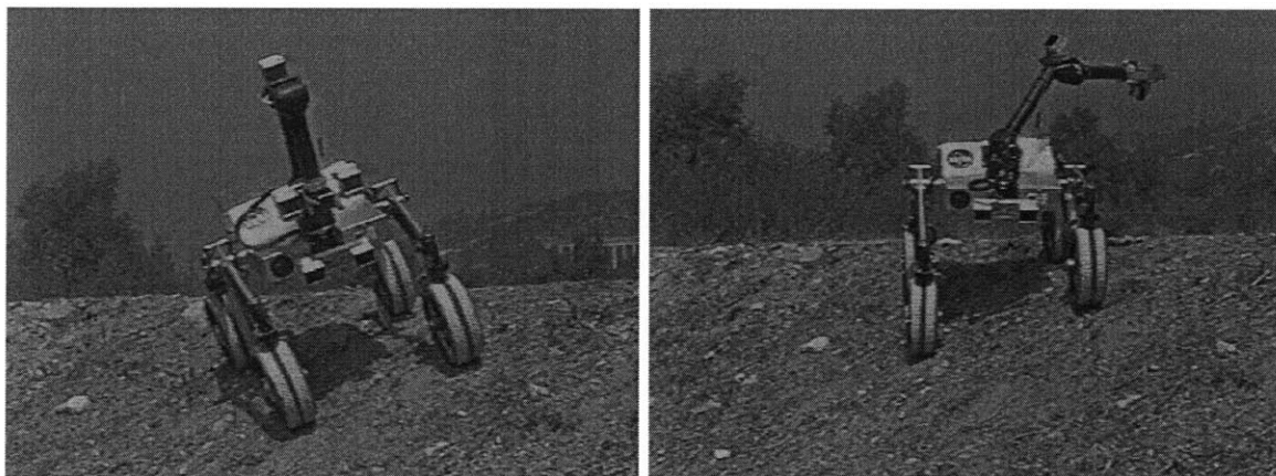
Figure 20: SRR experimental trials in the Arroyo Seco. Non-reconfigurable system (left), reconfigurable system (right).
