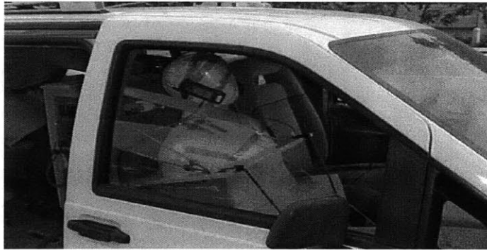
Figure 4-2: Measurement van with phantom head dummy
