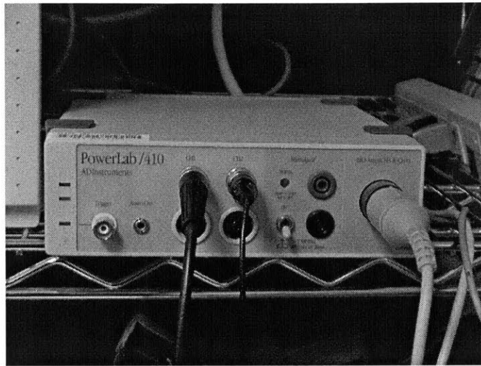
PowerLab 410, used for PPG vs. Pressure measurements
