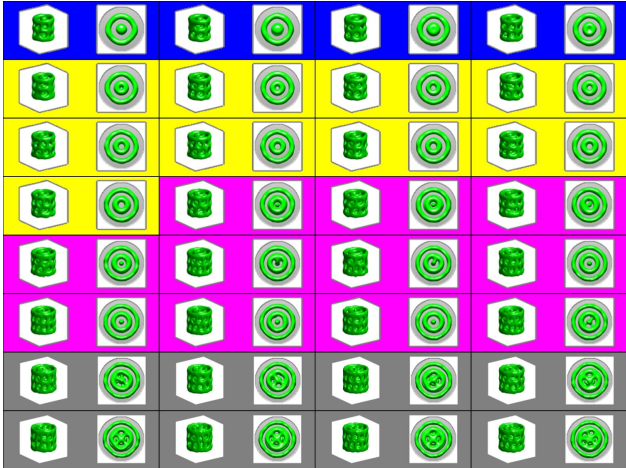
Figure 5-50: 3D simulation results of a 4L_0 thick hole of a cylindrically confined cylinder forming PS-PDMS with neutral top surface conditions and PDMS preferential surface conditions on the rest of the surfaces. From upper left corner to right and then down results are shown from d/L_0 = 4.0 to 6.6 . Left images are 3D side view with boundary conditions cut away and right images are top-down cut through views. General trends are for more concentric features to form as d/L_0 increases to different commensurations. Simulation parameters are \chi N = 18 and f = 0.36 . Plots are of \phi = 0.5 isosurfaces. Color coding is analogous to 2D results in Figure 5.44 only considering the top-down morphology appearance. The phase at the highest diameters (grey) was not observed in 2D simulations in terms of top-down views of 3D results where the ring in the center started having interconnections like confined perforated lamellae rings. Also, the double ring with single sphere phase (pink) had defects in different layers sometimes with the internal ring sometimes connecting to the internal sphere or cylinder going through the rings.
