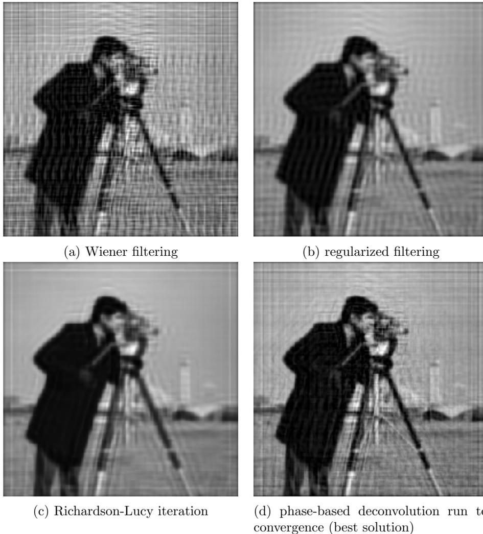
Figure 4-19: Cameraman image restored with several different methods when the blurring filter was an 11x11-point Gaussian with  $\sigma = 5$  and the deblurring filter was a 9x9-point averager
