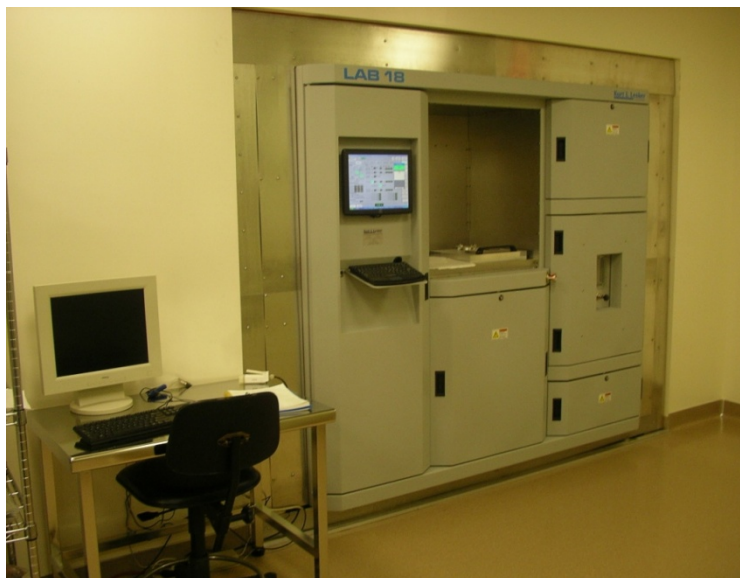
Figure 2.1 – Kurt J. Lesker Lab 18 sputtering system located in NanoPrecision Deposition Laboratory at MIT
