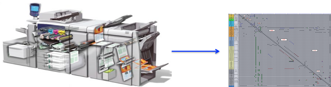
Fig. 5.15: Old Digital Printing System (Shown with High Capacity Feeder and Finisher) with its DSM (Size 91x91).
