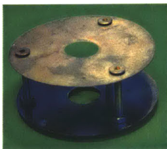
Figure 3.7 Heat shield for gold tube furnace
