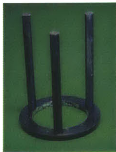
Figure 3.12 SS structure to support samples inside furnace
