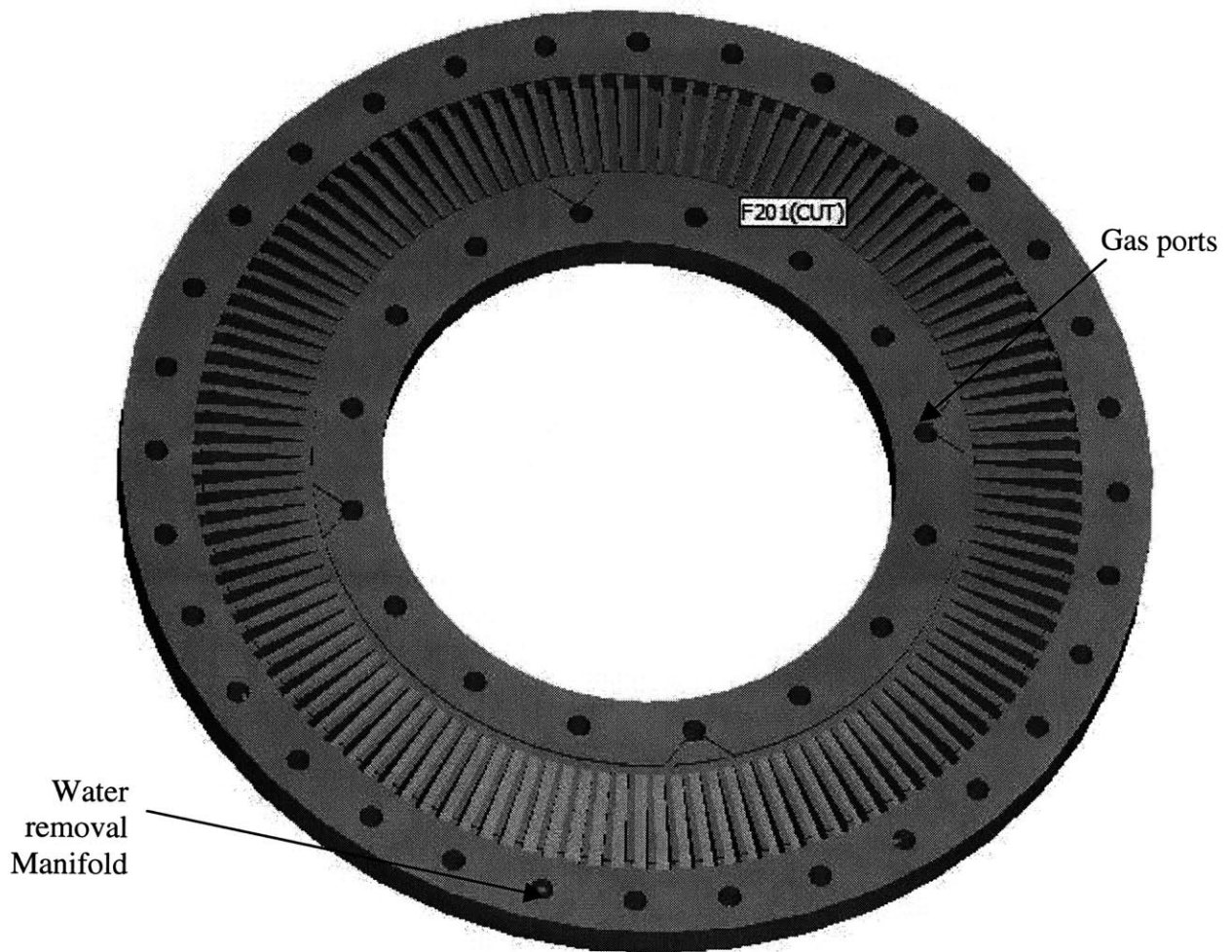
Figure 5: Top (oxygen side) of the bipolar plate
