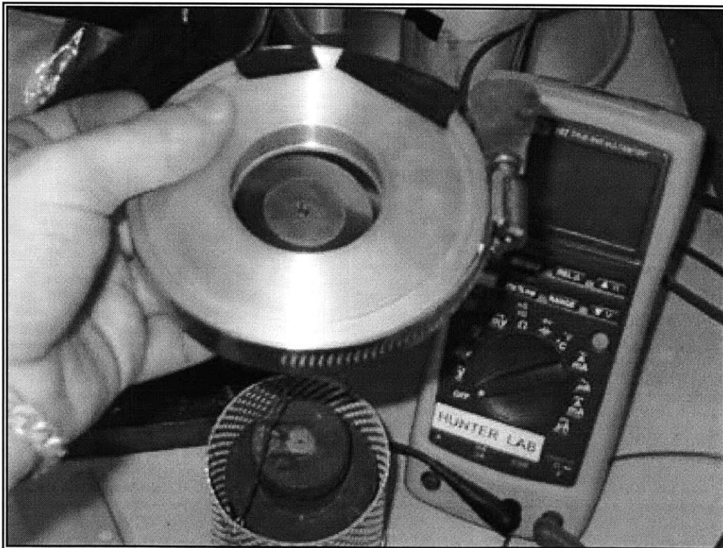
Figure 5.2: A brass plug is used as an anchor for the weight basket below as the valve disk is inserted into the aluminum mounting block
