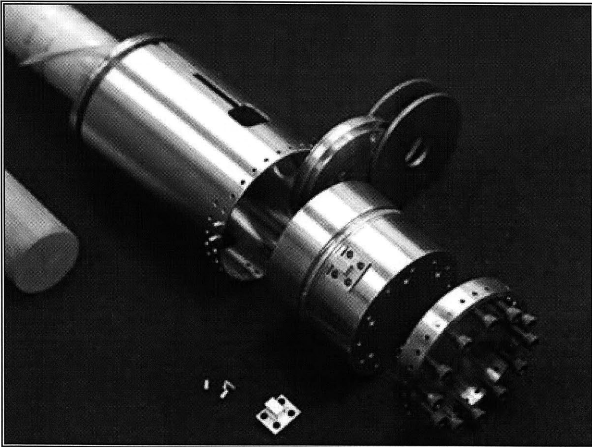
Figure 6.1: The cold end consists of several components that when assembled together support the function of the valves in the context of the larger machine
