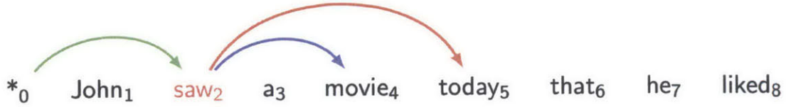
Figure 6-5: Example of a scored part in a grandparent/sibling model. The function \omega(h, t, s, m) looks at the head, grandparent, sibling, and modifier to produce a score. For this example the grandparent is *_0 , the head is saw_2 , the sibling is movie_4 and the modifier is today_5 .
