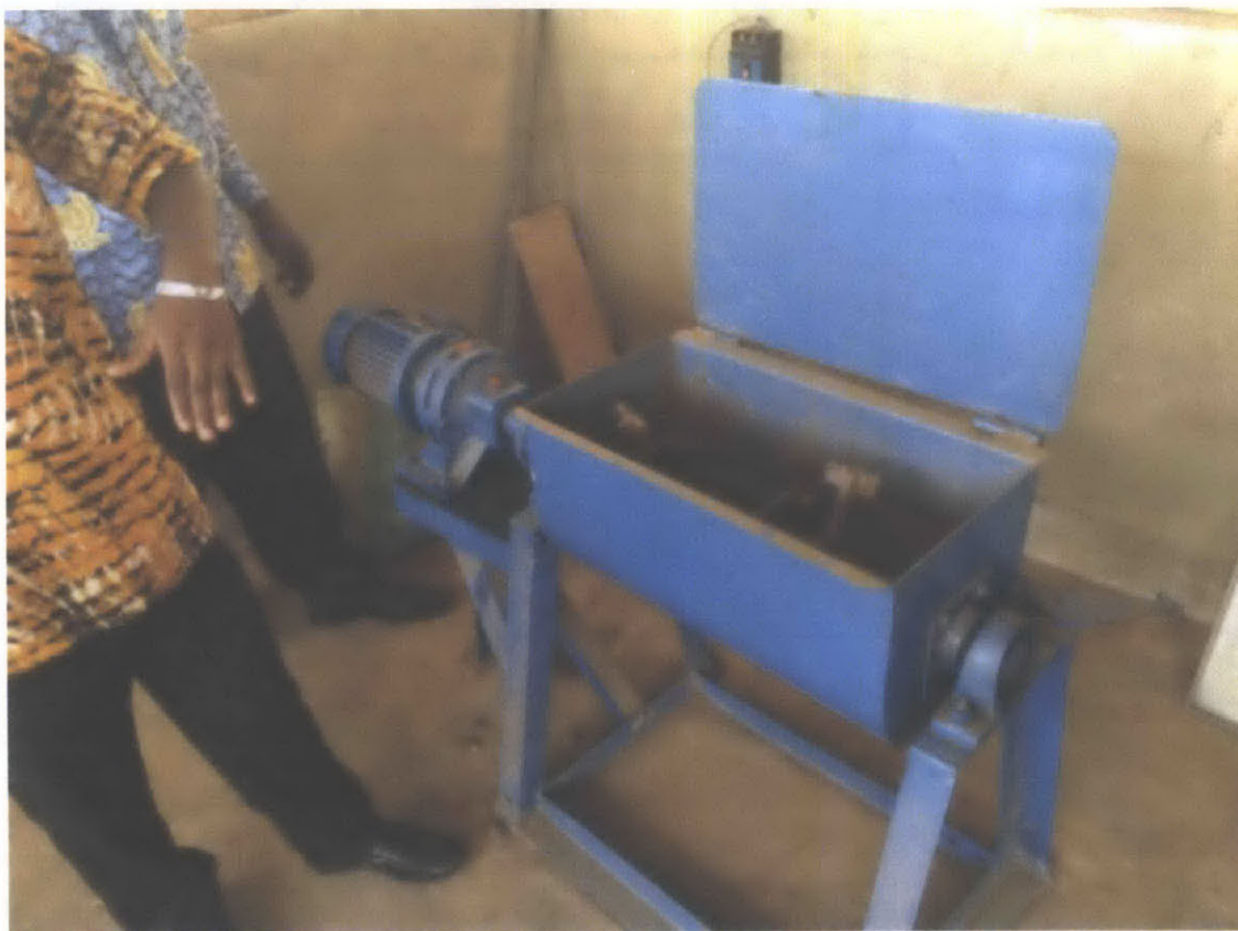
Figure 7-7 Inside the mixing machine, pictured above, inorganic fertilizer and pre-gelatinized cassava starch are mixed with the compost
