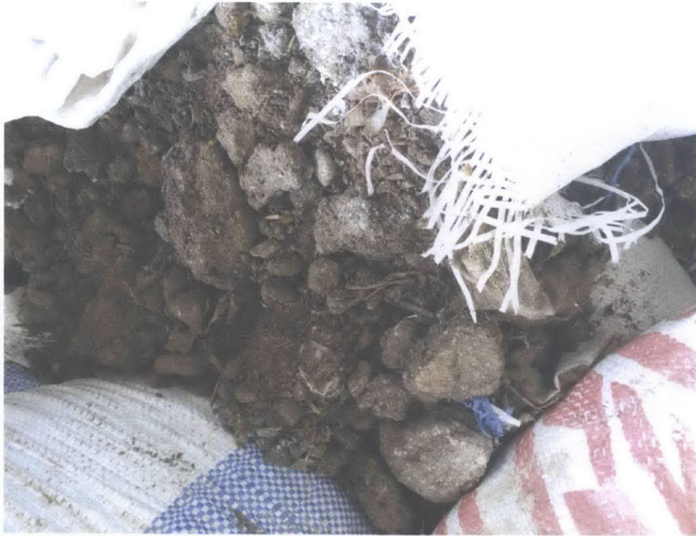
Figure 7-5 Raw dewatered fecal sludge, delivered from the drying beds at Tema
