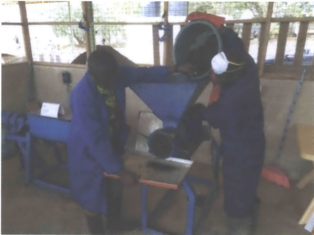
Figure 7-8 The final mixture of compost, inorganic fertilizers, and cassava starch is extruded to produce pellets for agriculture
