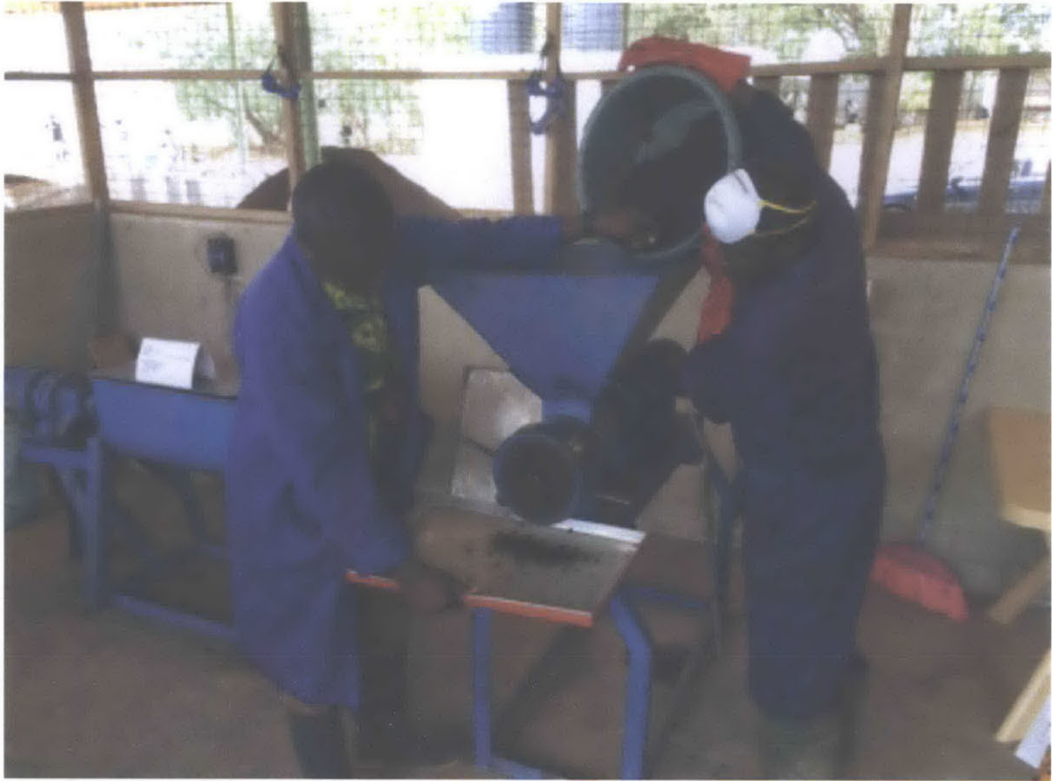
Figure 1-15 Two researchers produce fertilizer pellets from composted fecal sludge
