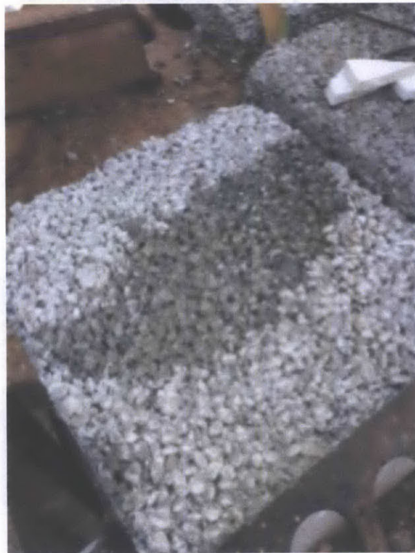
Figure 5-4 The permeable concrete filters used in Biofilcom's Biofil digestion tank
