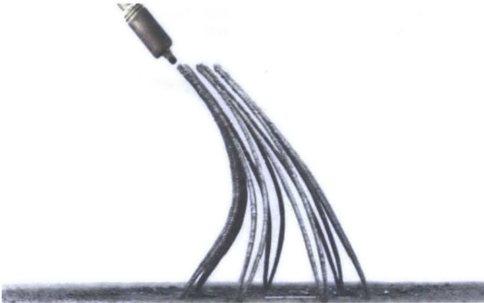
Figure 3 : Steel 3D printing at the Joris Laarman Lab in Amsterdam ( http://techxplore.com/news/2014-02-3d-metal-amsterdam-lab-video.html )
