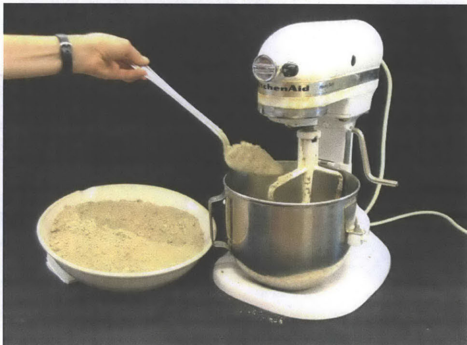
Figure 3-6: Mixing of clay powder and water into a slurry
