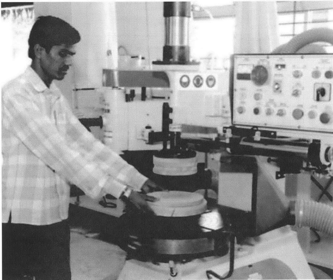
Figure 3-6: Example of Crafts Park Machinery- Auto Copy Shaper(Outer)
