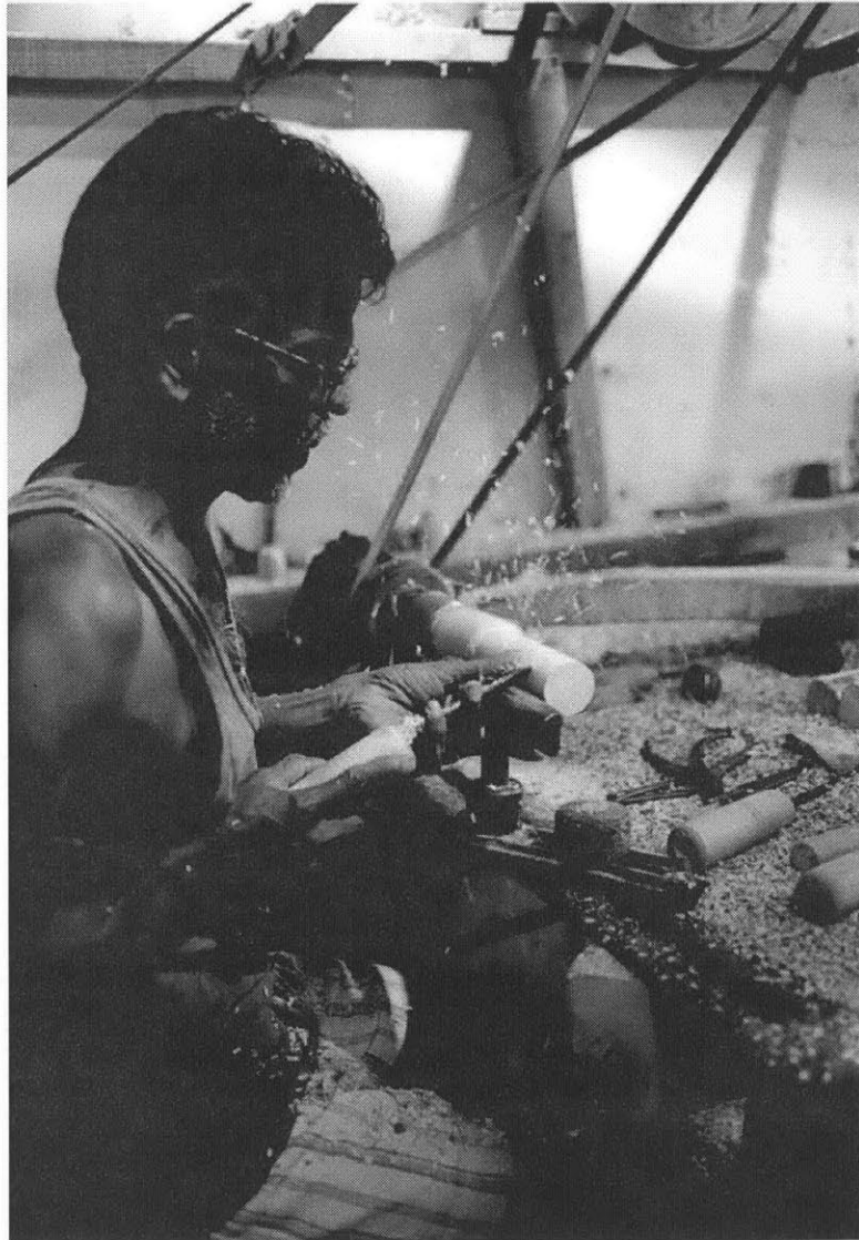
Figure 3-8: Technology Used by Artisans- Motorized Lathes and Hand Tools
