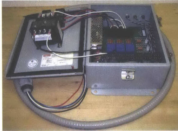
Figure 2-3: NILM Hardware enclosure
