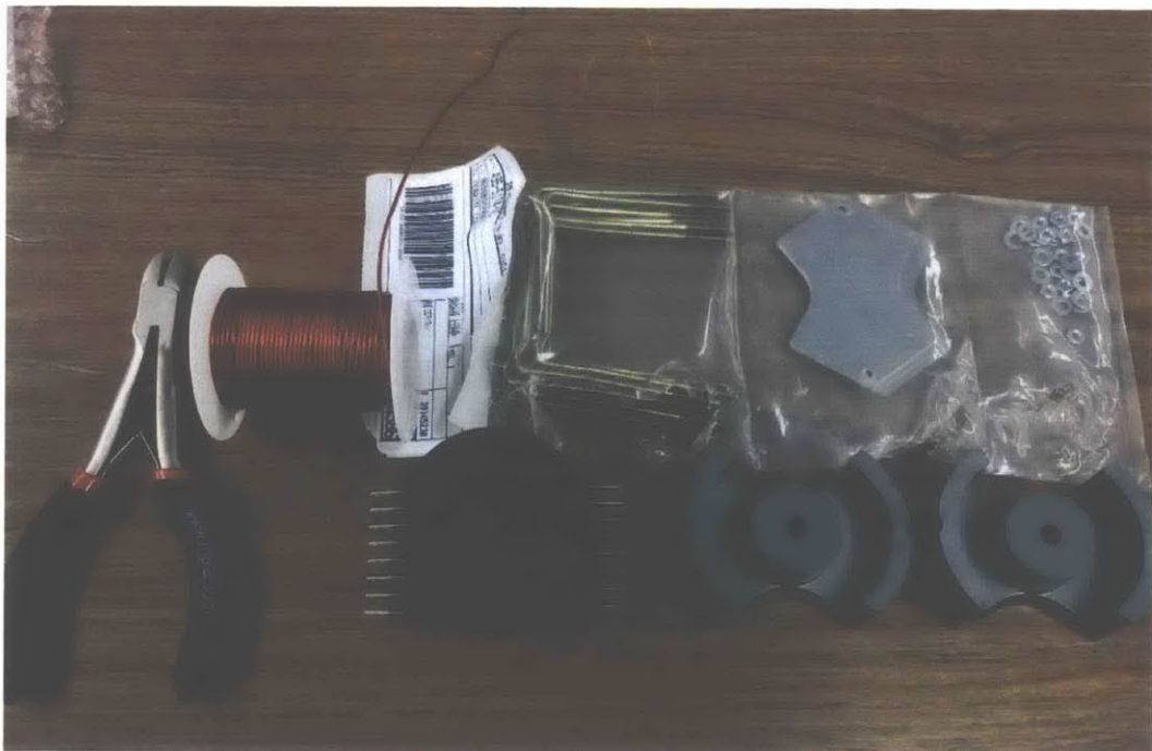
Figure 40. Inductor build materials: 16AWG coil, inductor core, and mounting assembly.
