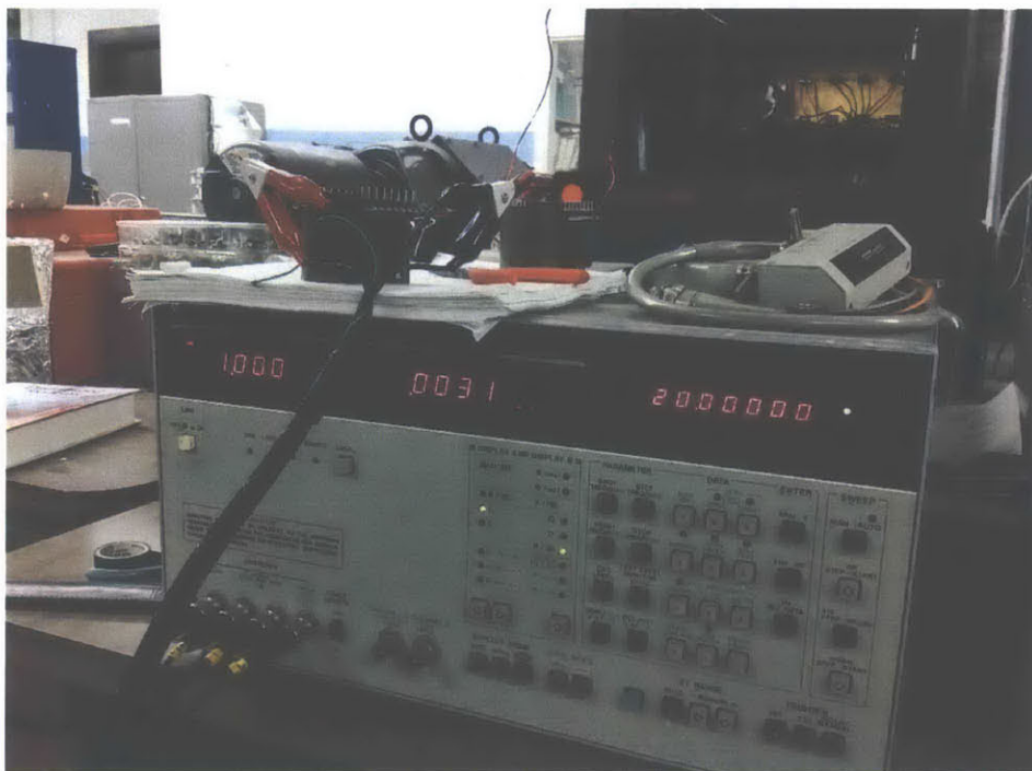
Figure 30. 1mH inductor and its inductance test.
