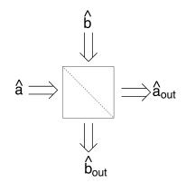
In last weeks homework you used and measured entangled states. This problem will demonstrate one of the ways experimentalists can create and manipulate such states using simple optics such as a beam splitter. An ideal beam splitter transforms two input field modes,  $\hat{a}$  and  $\hat{b}$ , according to
