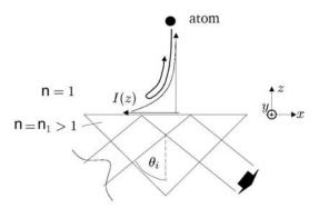
It is possible to construct an effective wall for atoms using dipole forces induced by light. A realization of such a wall is the short range repulsive potential formed by an evanescent wave. This wave is produced by total internal reflection of light at a dielectric interface. The interface is mounted horizontally and the atoms are dropped onto it.
