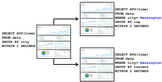
Figure 5: A possible root-cause analysis scenario for detecting the cause of latency spikes in Kensington.
