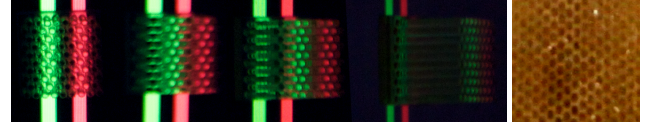
Fig. 4. Air cladding fibers have 180 degree field of view and excellent transmission, but they are impractical since support material is added between the fibers during printing. This support material is very hard to clean for the intricate fiber geometries used in this work. From left to right, we see light imaged from increasingly grazing angles. On the back, a laptop screen feeds light into the bundle. At extreme right, we show the hexagonal cross-section at the base of our fibers. This shape improves tiling of the input image plane with no observable loss in fiber transmission.
