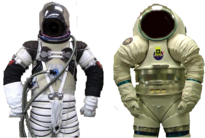
Figure 2.3. Advanced concept space suits for technology demonstration. A) The David Clark Demonstrator suit. Photo credit (Jacobs 2011) B) The Mark III designed for planetary exploration and mobility.
