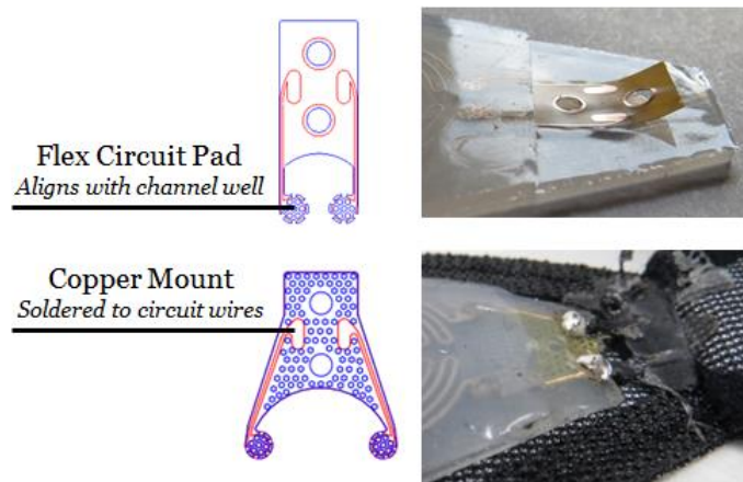
Figure 4.4. Flex circuit components and improvement features over previous designs. Copper coated kapton is chemically etched (outline in red) to create the circuit pathway from the pad to the mount. Laser cut perforations (outline in blue) allows for better mating between sensor halves and improves durability. Pads were separated to prevent leakage under pressure.
