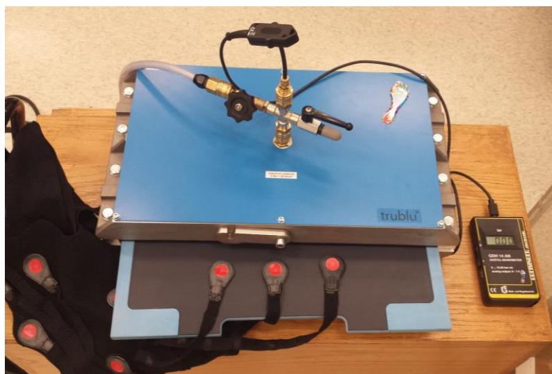
Figure 4.5. Calibration apparatus. Sensors loaded with constant pressure at 10 kPa increments from 0-60 kPa. Pressure measured with manometer with resolution of \pm 1 kPa.
