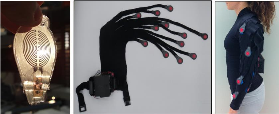
Figure 6.2. Each component of the Polipo pressure sensing system. The pressure sensors are molded with a silicon elastomer filled with an electrically conductive liquid metal, gallinstan. The sensors are integrated to a wearable electronics system designed for the 50 th percentile female to the 95 th percentile male in upper body dimensions. The system takes into account the unique environmental of the space suit allowing for over 4 hours of continuous pressure measurement between the space suit and person’s arm during dynamic movement.
