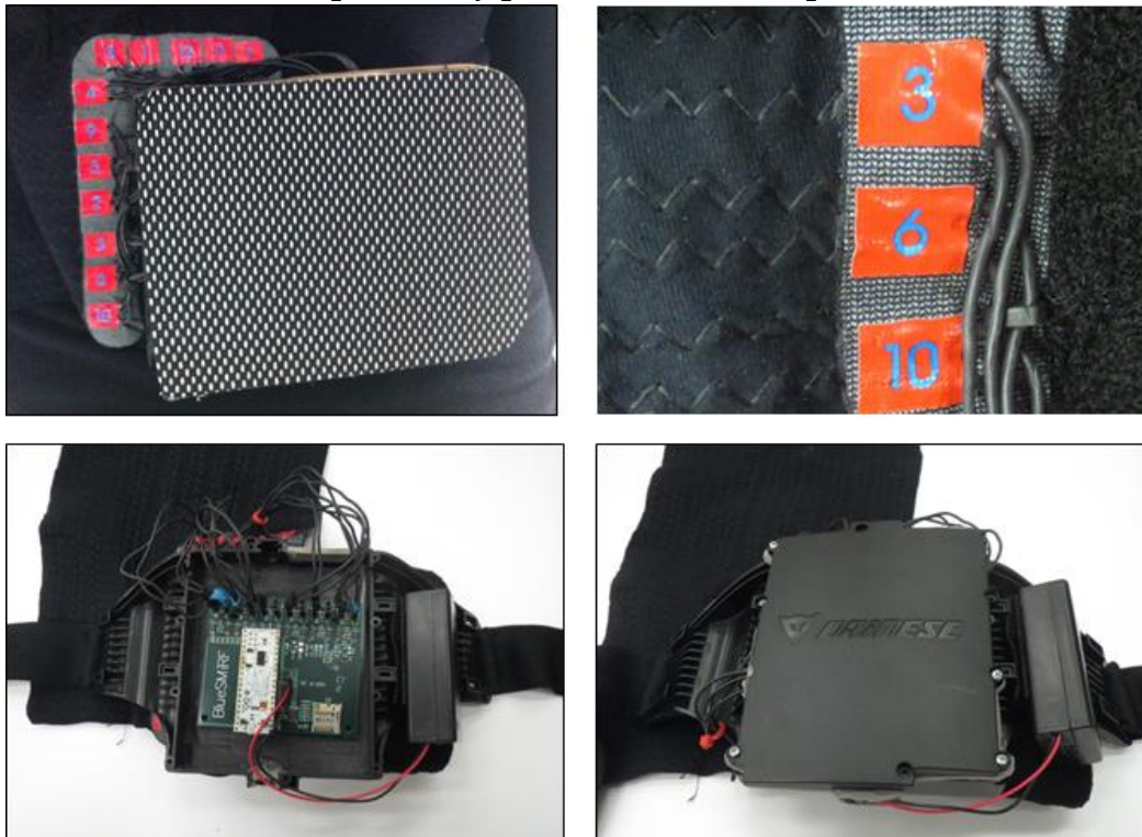
Figure 4.16. Electronics housing and configuration. A) The deformable electronics box with sensor wiring, B) The transition from the elastic wires to the input into the electronics boxes are labeled by sensor. C) The electronics board was custom designed with 12 sensor inputs collected with an Arduino Micro and stored on a micro SD card. D) The smaller profile electronics box and battery mount. This is the configuration used for human-space suit testing.
