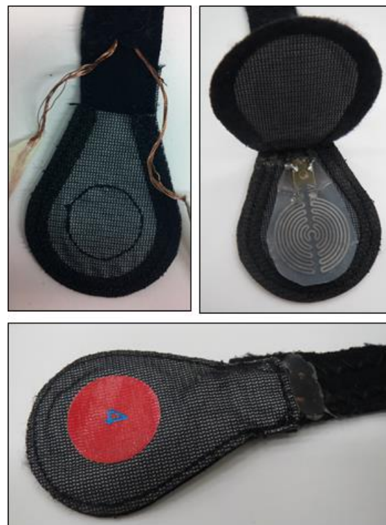
Figure 4.14. Components of the Chele. A) Open view of the chele with bare wires B) Sensors are soldered into place and wires are fixed and isolated, C) Final configuration with sensor integrated.
