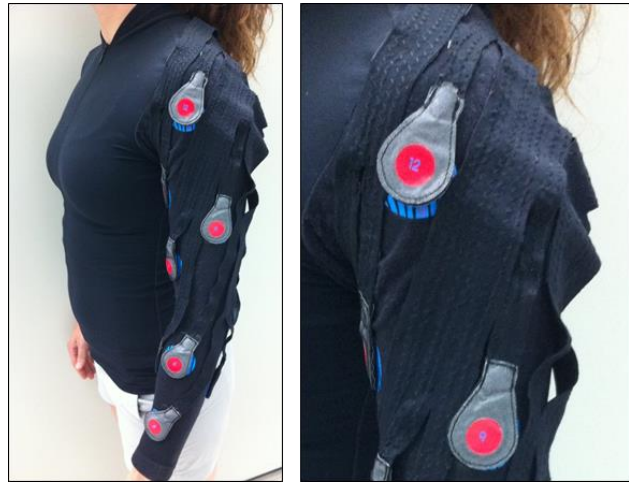
Figure 4.18. Final design of the Polipo pressure sensing system worn on the body. An additional layer (not shown) is worn over the system to prevent the wires from catching or sensors moving.
