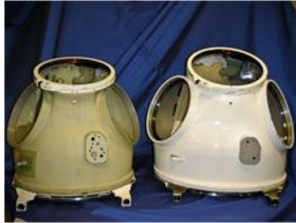
Figure 2.2. Pivoted and planar hard upper torso (HUT) styles. There are two HUT styles with their primary difference being the shoulder scye bearing to which the arm components attach. The pivoted HUT, shown on the left, has a pivoting bellows to allow for greater shoulder mobility than the planar HUT, shown on the right. Photo credit NASA.
