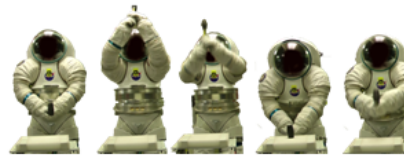
Figure 5.4. Movement tasks performed by each subject. Three isolated joint tasks are performed: Elbow Flexion/Extension, Shoulder Flexion/Extension, and Shoulder Abduction/Adduction. Two functional tasks were performed: Cross Body Reach and Overhead Hammering. Subjects were given very specific instructions on how to perform the isolated joint tasks, while subjects were given way-point markers to meet and allowed to develop their own biomechanical strategies for the functional tasks. Subject suited in Mark III suit is shown.
