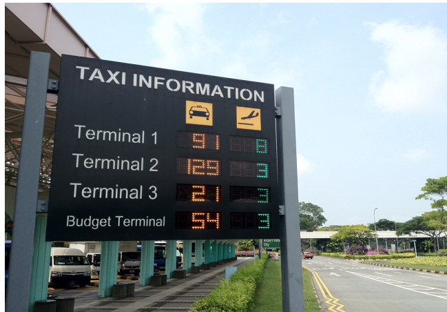
Fig. 1: Electronic signboard on the highway leading to Changi Airport showing the number of taxis at each terminal, along with the number of flights arriving in the next half hour.
